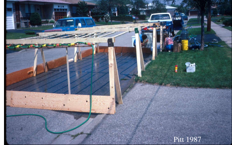
Street dirt washoff and runoff test plot, Toronto
